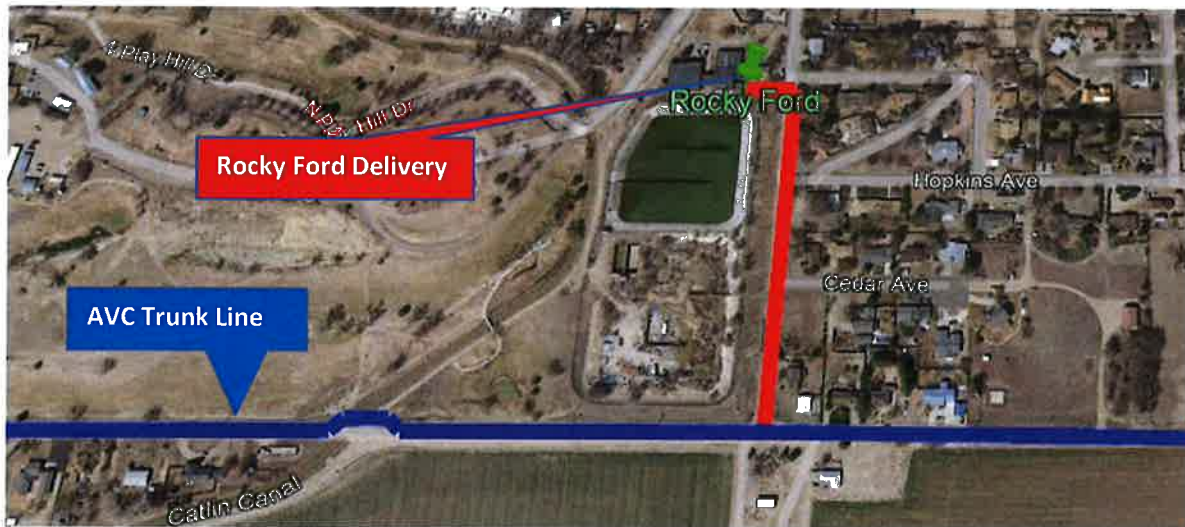
MAP 4: The Rocky Ford delivery line will be about 0.2 miles from the trunk line to the water plant.
